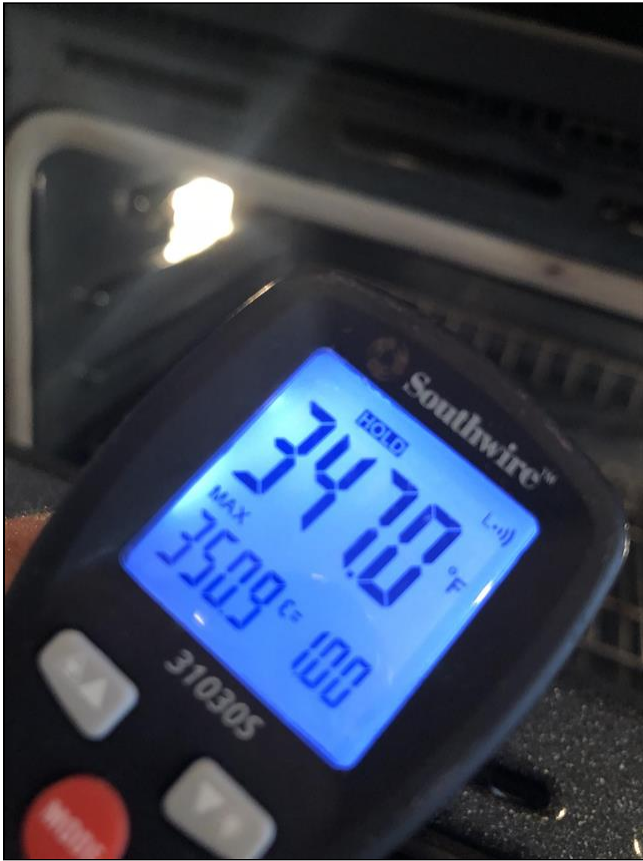
10.1 Item 3(Picture) Upper Oven Temp
