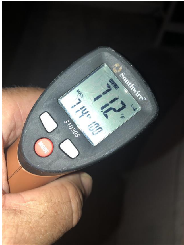
8.8 Item 10(Picture) Return Air Cooling Temp
